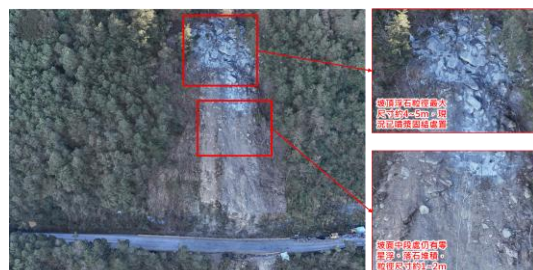
圖 11 無人機建模浮落石料源判釋成果 Figure 11 UAV-based modeling results for identifying loose rockfall sources
