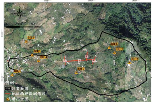
圖 5 地球物理探測測線及鑽孔位置分佈圖 Figure 4. Geophysical survey line planning and borehole location distribution map
