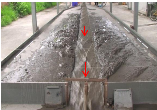
圖 16 試驗後期沖淤情形 Figure 16. The Flushing Condition in Late Stage of Experiment
