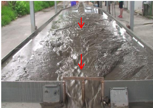
圖 15 深槽冲刷與側灘淤泥崩落現象 Figure 15. The Flushing Condition of Deep Grooves and Silt slide from Beach
