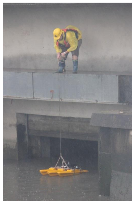
圖 6 ADCP 搭配小型載具進行閘門流量觀測 Figure 6 Observing gate flow by ADCP on a boat.
