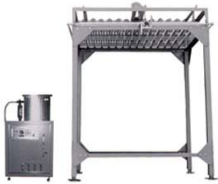
圖 2. 人工降雨器設備(Daiki Rika Kogyo Co.,Ltd) Figure 2. The equipment of rainfall simulator.
